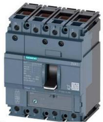
CIRCUIT BREAKER 3VA1 IEC FRAME 160 BREAKING CAPACITY CLASS S ICU=36KA @ 415 V 4-POLE, LINE PROTECTION TM220, ATFM, IN=160A OVERLOAD PROTECTION IR=112A ...160A SHORT CIRCUIT PROTECTION II=10 X IN NEUTRAL UNPROTECTED CABLE CONNECTION
